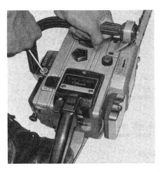
Pull the rope 5 or 6 times, and the engine will emit the first firing sound. Then push the choke button back to the original position. Next, pull the rope, and the engine will start.
