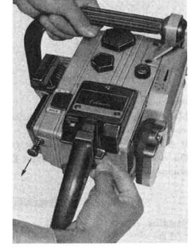
\* Before pulling the recoil starter rope, be sure to hold the chainsaw firmly on the ground by the foot.
